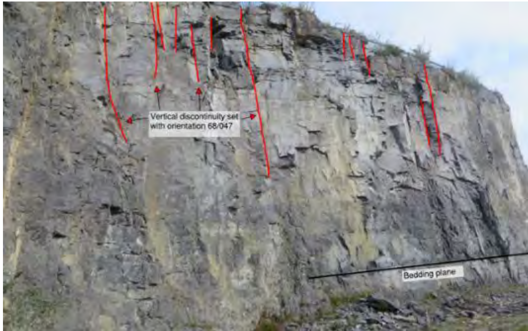
Figure 3.17: Exposed discontinuities on the upper bench
