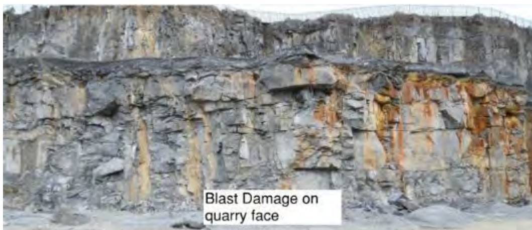
Figure 3.18: Blast damage on quarry face
