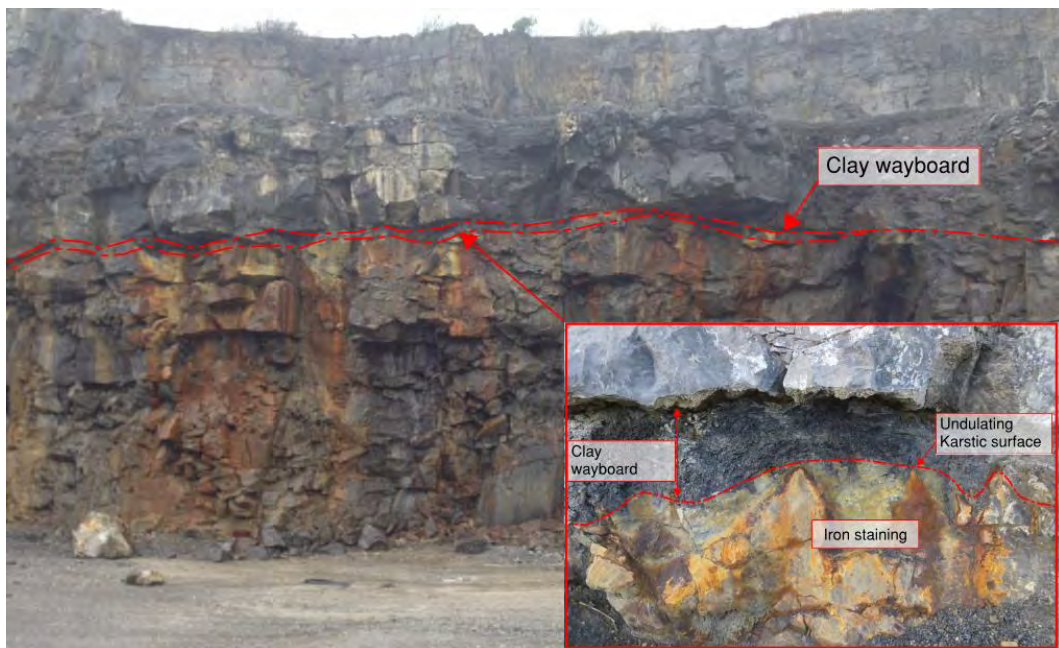
Figure 3.16: Clay wayboard on the quarry face at Lackagh Quarry
